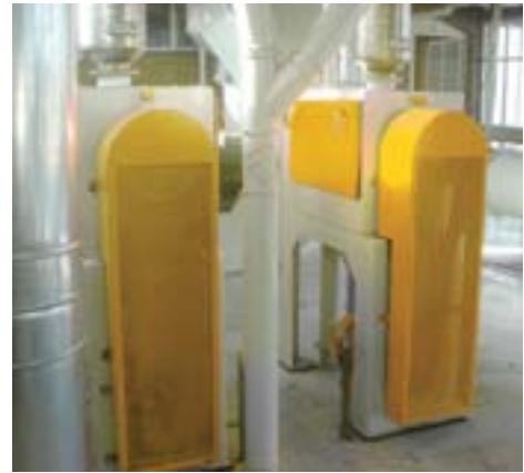
Bran finishers (or Bran dusters) are used to separate the flour sticking on the bran generally after the lower break scalpers of mill streams. Optimum results are obtained by treating the coarse and fine overtails separately.
