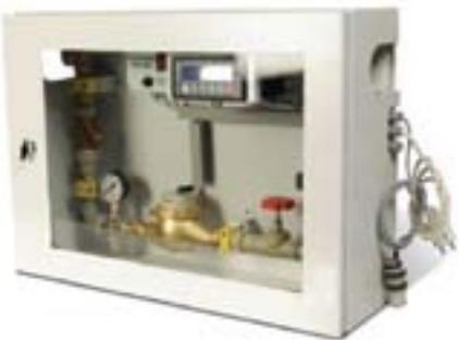
Digital screen flow meters transmit the data received from the flowing grain by the capacitive sensors placed in the entrance of the product entry of the dampeners. They count the pulse data received from the digital water meter on the flow meter, shows how much water flows per hour and stores the value in the memory. They also produce an output of 4 – 20 mA, and by evaluation of this data in its PLC; flow can be observed from the PC, too.
